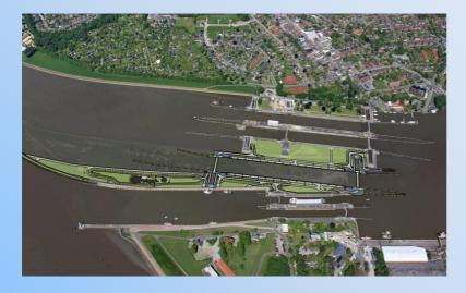
The present sluice complex at Brunsbüttel comprises the two twin locks, each, of the small (old) lock in the south and the large (new) lock in the north of the complex.
